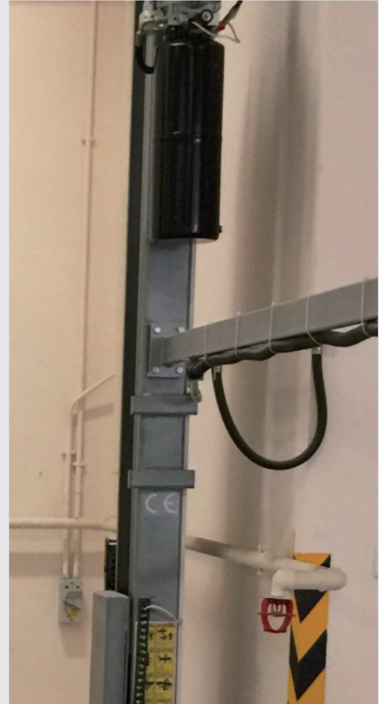
Two position locks only stop platform in the top.
